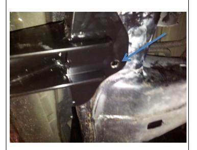
20. Bend M12 cage nut plate so it can be inserted into chassis rail .Align with the square hole in the bottom of chassis rail and start M12 x 40 bolt with spring and flat washers.(RHS shown)
