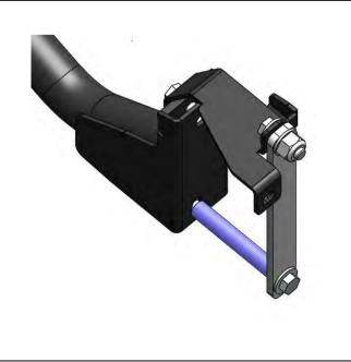
22. Insert the rear fixing plate underneath the pipes on the inside of the chassis then attach to the top bracket finger tight only, using an M12 x 40 mm bolt, nyloc nut and flat washers as shown.
