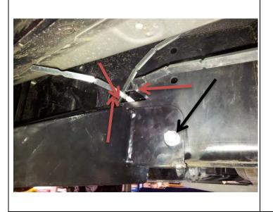
19. Bend 2 x M8 nut plates so they can be inserted into chassis rail .Align these with the 10mm holes in the side of the rail and start M8 x 40 bolts with spring and flat washers .Trim tabs with side cutters at red arrows to insure tabs do not rattle on chassis.(RHS shown)
