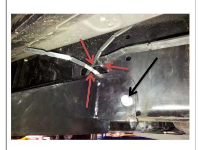
30. Bend 2 x M8 nut plates so they can be inserted into chassis rail. Align these with the 10mm holes in the side of the rail and start M8 x 40 bolts with spring and flat washers. Trim tabs with side cutters at red arrows and insure tabs do not rattle on chassis. (RHS shown)
