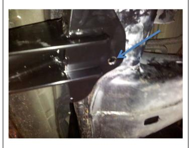
31. Bend M12 cage nut plate so it can be inserted into chassis rail. Align with the square hole in the bottom of chassis rail and start M12 x 40 bolt with spring and flat washers.(RHS shown)
