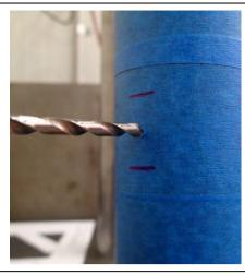
25. At the location of the Centre Punch mark, use an Ø4mm (or similarly sized) Drill Bit to drill a pilot hole through the front face of the Bull Bar outer frame.
